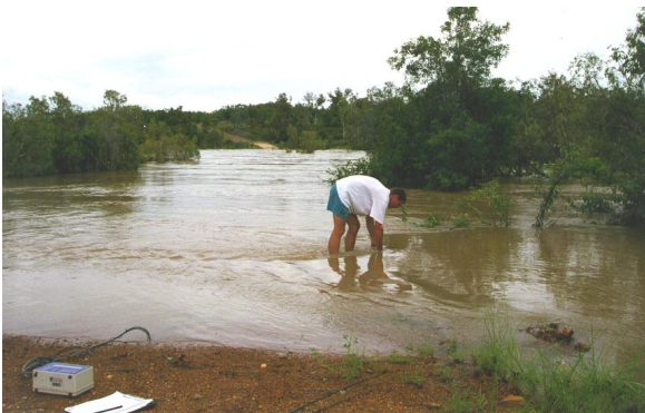
Figure 5 Obtaining water quality information using an electronic datalogger and by collecting a water sample for laboratory analysis. Photo courtesy of: Mitchell River Water and Environmental Quality Project
